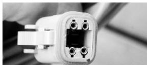
4. Install the wedgelock into the face of the connector. It will click into place.
