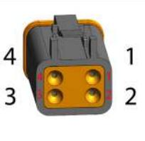
3. Inspect the receptacle from the face of the connector. The receptacles should be flush with the face of the connector
