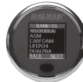
The currently selected battery type is noted with an asterisk (\*) in front of the name. The default is AGM-STD (see the chemistry table). If this is your chemistry and the installation is new, you may either re-select the chemistry, ensuring that the SG200 is starting fresh, or exit back to MENU and move to the next step.
