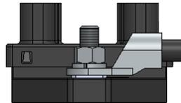
6. Connect the voltage sense leads to the auxiliary batteries. AUX-1 is a solid orange wire, and AUX-2 is orange/black. Each AUX lead needs to be fused within 6" of the battery. Fuses MUST BE INSTALLED FOR THESE WIRES, and are not included. The wires do not carry any current, so the fuse should be sized for the wire gauge and length. If you need to extend the wire, do so with at least 18ga wire.
