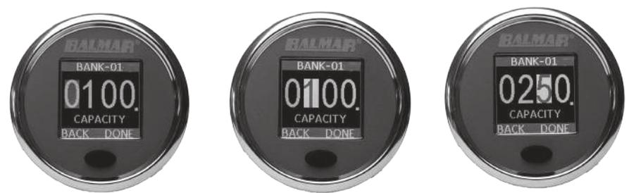
Once you select a chemistry, you must specify the capacity of the battery bank. This is the total design capacity of the entire bank, regardless of the battery's condition, or previously measured capacity. Typically the capacity is expressed as the 20-hour discharge rate. This may be written as something like "105Ah/20h" on the battery or battery documentation. If you cannot find an Ah specification for your battery, but it does show a reserve capacity (RC)
