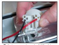
Strip approximately 3/8" of insulation off of wires and insert wire ends into the bulb recepticle. Wires will be locked in once completely engaged. Note that four wiring connectors are supplied on the bulb recepticle for multiple light circuits.
