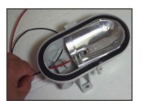
2Punch out the required number of wire holes required for installation. Three holes are provided. Holes are scaled for 1/2" conduit. Insert positive and negative wires.
