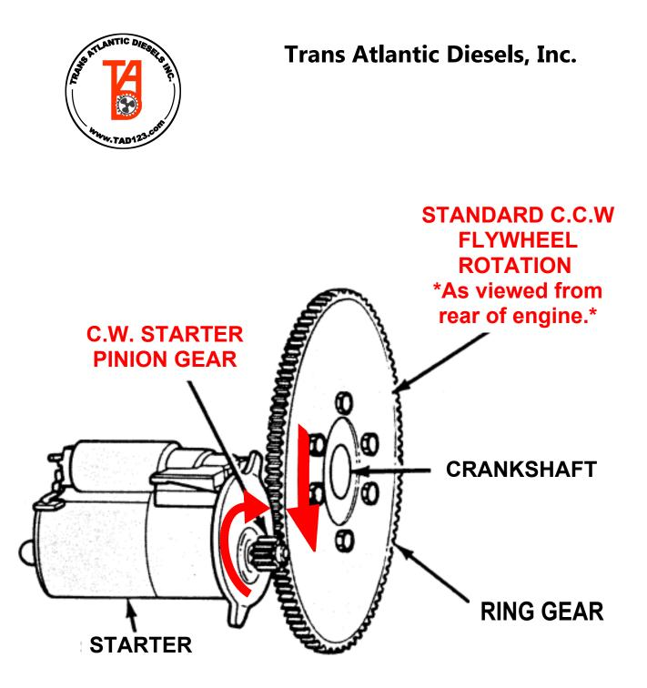
A C.W. (Clockwise) rotation starter drives a C.C.W. (Counter-Clockwise) rotation flywheel as viewed from the engine rear. (As shown above)
