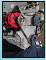
For 200 amps 12v the New Balmar AT-200 Alternator is a great choice. This unit has a very impressive performance curve and is particularly well suited to high output at low speeds. (Performance curve attached.) TAD offers the 200 amp alternator as a complete kit with MC614 Smart Regulator, wiring harness and temp alarms for battery & alternator.
