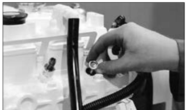
**Figure 17:** Remove and replace copper sealing washer.
