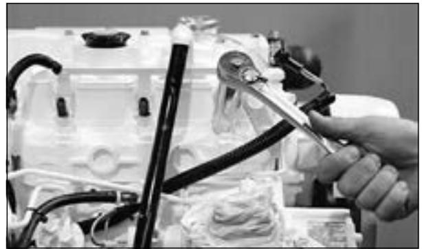
**Figure 16:** Unscrew injector.
