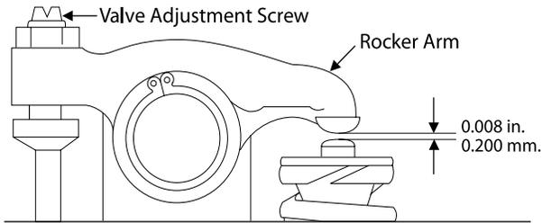
**Figure 8:** Valve Adjustment
