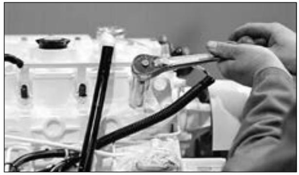
**Figure 18:** Reinstall injector. Torque to proper tightness.
