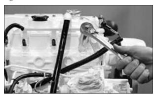
Figure 16: Unscrew injector.
