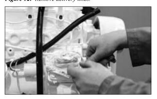
Figure 13: Cover lines, inlets and injection pump outlets.
