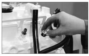
Figure 17: Remove and replace copper sealing washer.
