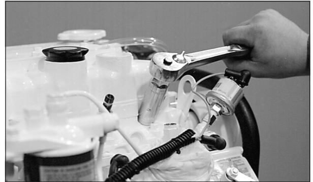
*Figure 18: Unscrew injector.*
