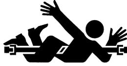
Do not wear loose fitting equipment around rotating drivelines. Stop the engine and make sure that all moving parts have stopped before making any adjustments, connections, or performing any other type of service to the engine or other driven equipment.
