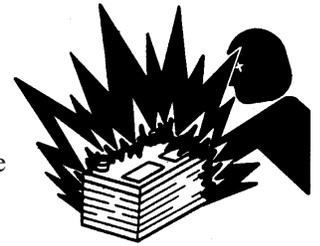
Frozen batteries may explode if charged. Never charge a battery that has not been allowed to warm to at least 16°C (60°F).
