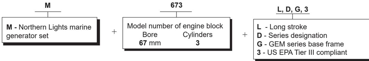
**M673LD3** = Northern Lights marine diesel generator set with a 673 engine long stroke, TF-276D generator end US EPA Tier III, 5 kW.
