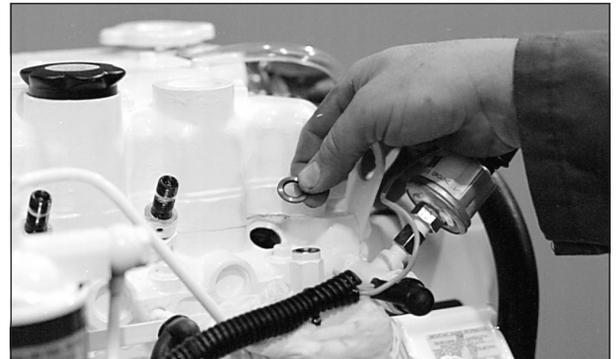
*Figure 19: Remove and replace copper sealing washer.*
