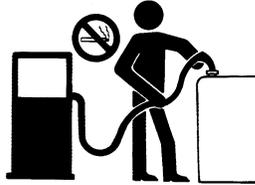
Prevent fires by keeping machine clean of accumulated trash, grease and debris. Always clean any spilled fuel as swiftly as possible. Do not store oily rags, which can ignite and burn spontaneously.
