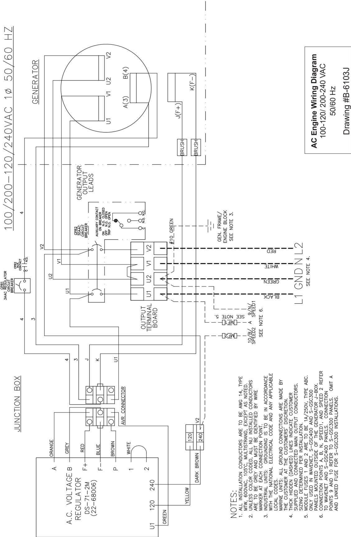
**AC Engine Wiring Diagram**
