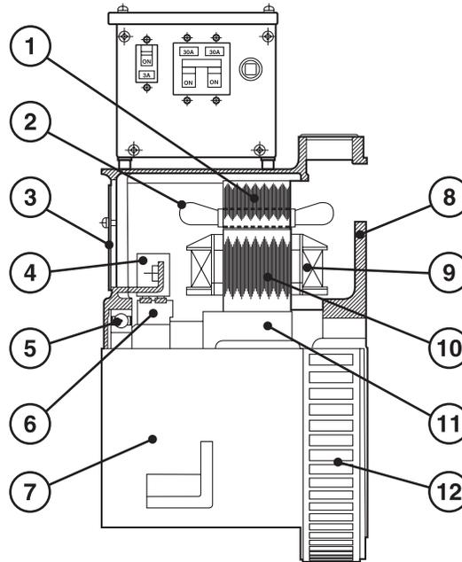
Figure 24: Generator Components.
