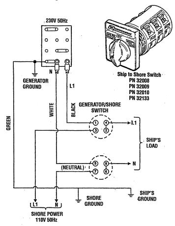
**NOTE:** Diagram shows connections for a two-wire, 120 volt system. For a three-wire system, use the dotted lines for the other hot leg.
