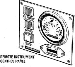
**PREHEAT:** The PREHEAT rocker switch/serves two purposes: activates the preheat circuit and activates the K2 Run Relay. This supplies power to the DC alternator **R**, fuel pump, ECU, Instrument panel, K3 Fault Relay pin #87 and Start toggle switch.
