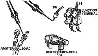
Windings Group C-2: The resistance value is measured between the lifted lead #1 from the Junction Terminal or Red Isolation Post below the transformer and lead #3 lifted off the AC Terminal Block. To totally isolate this winding group. Lift lead #2 off the terminal Block.
