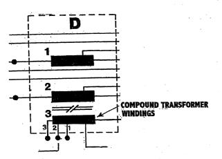
**Transformer Auxiliary-Windings D-3:** Remove all three leads **#1, #2,** and **#3** from the three position terminal strip (located just below the transformer). Lift the black and green leads from the AC terminal block and measure between red **#1** and the black lead. Transformer Auxiliary Windings Resistance
