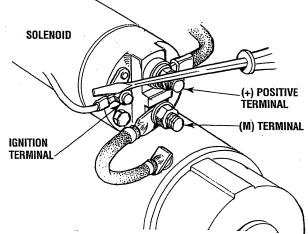
**If nothing at all happens the solenoid isn't getting current.** Check the battery isolation switch and inspect the wiring connections. It is also possible that the solenoid is defective.
