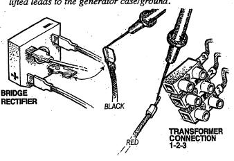
TESTING THE BRIDGE RECTIFIER (meter FLUKE multimeter)
