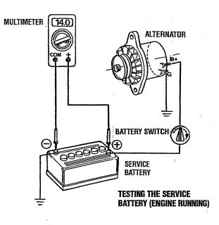
**A CAUTION:** When performing tests on the alternator charging circuit do not use a high voltage tester (i.e. Megger). You can damage the alternator diodes.
