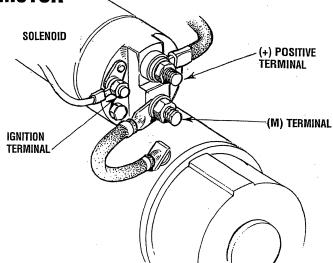
To test the ignition circuit, locate the ignition(s) terminal (it is one of the small terminal studs and is wired to the ignition circuit). Use a screwdriver, don't touch the blade, to jump from that ignition terminal to the positive battery connection terminal on the solenoid.
