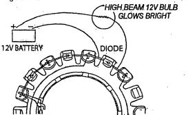
When leads are put across the diode, as illustrated, voltage passes through the diode allowing the headlight to glow brightly.
