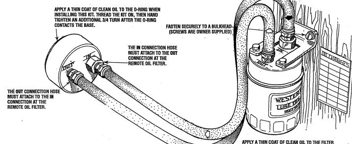
APPLY A THIN COAT OF CLEAN OIL TO THE FILTER Gasket when installing. After the filter Contacts the base, tighten it an additional
