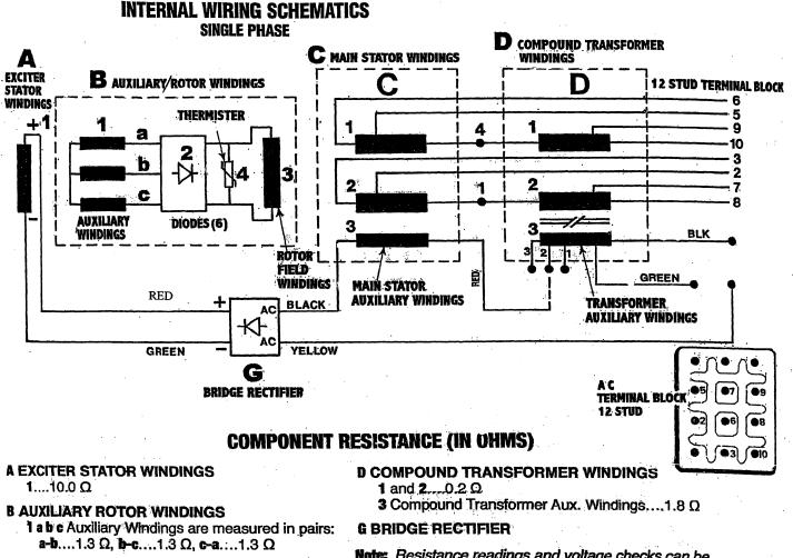
2 Diodes (6)....Ω/infinite
