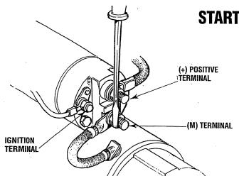
Test again by jumping the two large terminal studs. Hold the screwdriver blade firmly between the studs. Do not allow the screwdriver blade to touch the solenoid or starter casing, this would cause a short.
