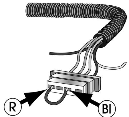
The regulator is now bypassed. When the ignition is engaged and the motor is started, the voltage should rise and charging current should be present.
