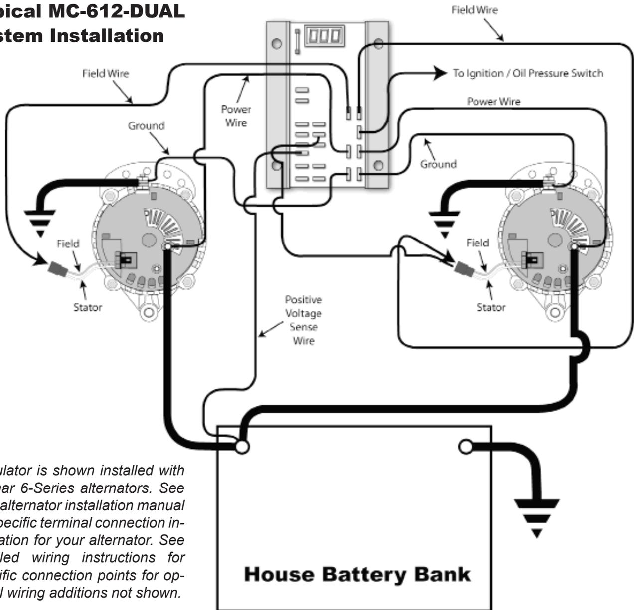
*Regulator is shown installed with Balmar 6-Series alternators. See your alternator installation manual for specific terminal connection information for your alternator. See detailed wiring instructions for specific connection points for optional wiring additions not shown.*
