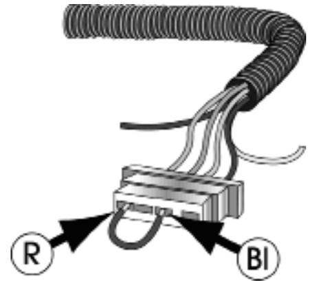
Testing the actual output of the alternator is known as “Full Field Testing”. This can be accomplished by jumping a positive 12VDC current to the field terminal at the rear of the alternator. This test eliminates both the regulator and the harness, making it easier to isolate your investigation to the alternator.
