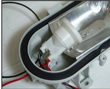
**4** Once the desired number of wires are connected to the bulb receptacle, snap the wired receptacle into the fixture's base. Screw a properly sized bulb in the socket (see page 1 for details). Install lens and guard.
