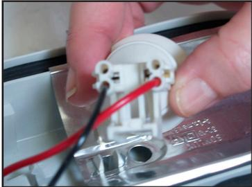
**3** Strip approximately 3/8" of insulation off of wires and insert wire ends into the bulb receptacle. Wires will be locked in once completely engaged. Note that four wiring connectors are supplied on the bulb receptacle for multiple light circuits.
