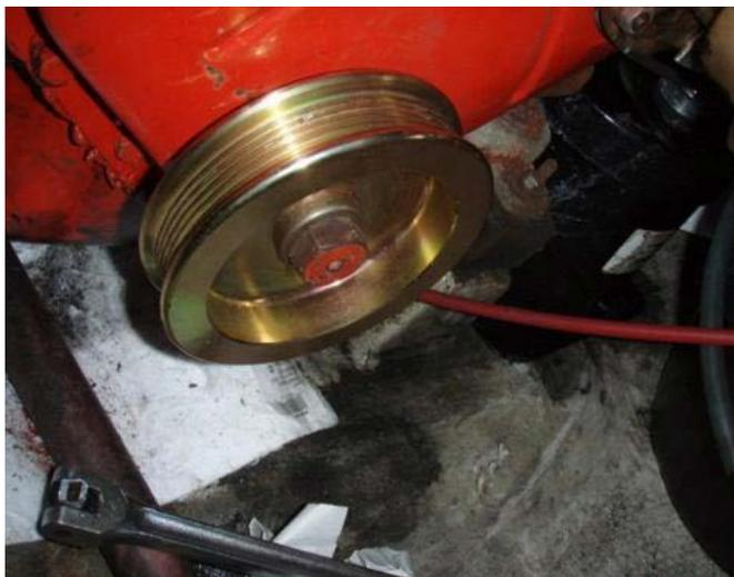
11. Completed serpentine crank shaft pulley.
