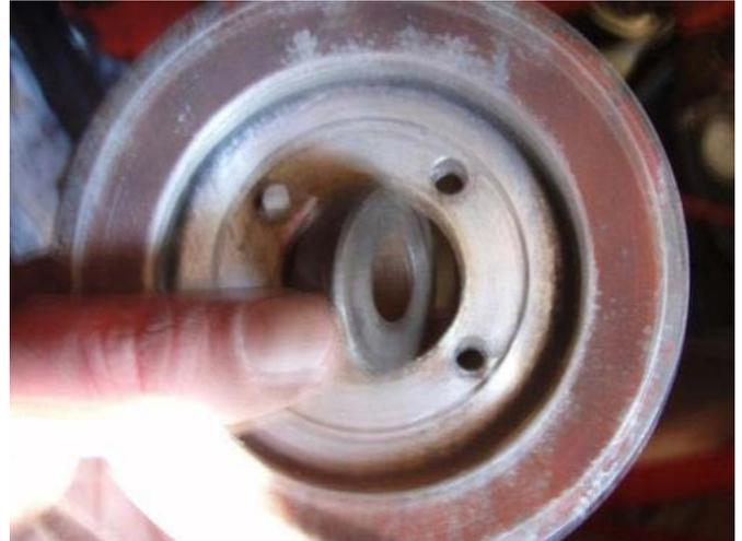
8. Remove the pulley washer from the old crank pulley and insert on the center crankshaft bolt.
