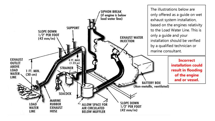
Figure 1. Properly installed wet exhaust system.
