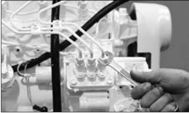
Figure 10: Remove delivery line flare nuts.
