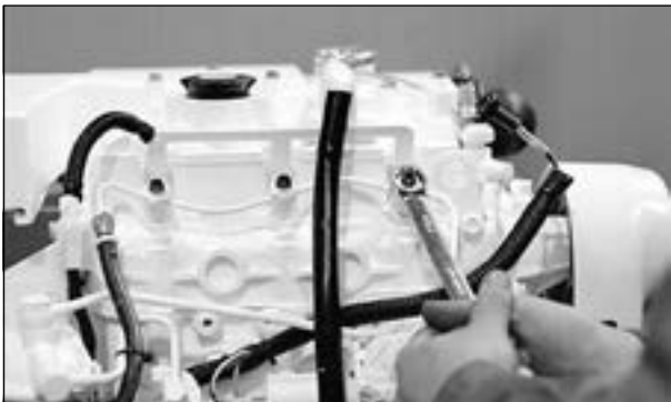
Figure 13: Remove return line nuts.
