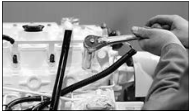
Figure 17: Reinstall injector. Torque to proper tightness.
