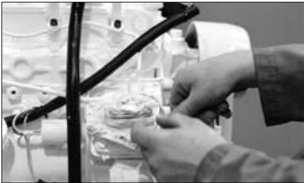
Figure 12: Cover lines, inlets and injection pump outlets.
